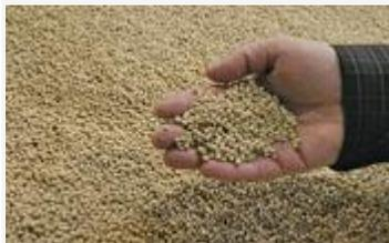
TRUEARTHGREEN's newest developments are focused on injection molding grades and have expanded its slate of wood polymer composites to include four polymer bases—polypropylene, polyethylene, HIPS, and TPO—as well as four fiber choices: pine, oak, maple, and rice hulls. Potential applications include automotive, consumer goods, toys, and construction.
