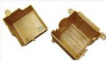
*WPC parts molded in a family tool designed for ABS/PC.*
